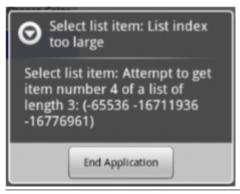
**Figure 19-9.** The error message displayed when the app tries to select a fourth item from a three-item list
